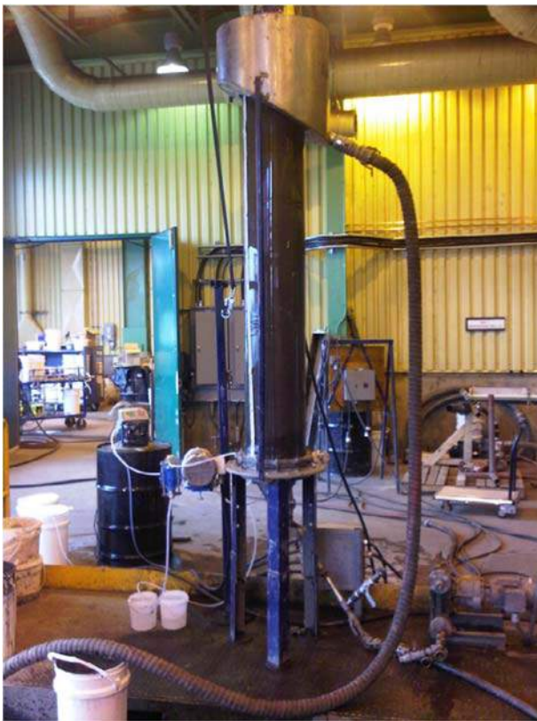
Figure 4. Photographs depicting the processing of Titanium’s fine fluid tailings in a thickener and rim ditch process at CanmetENERGY’s tailings testing facility.
