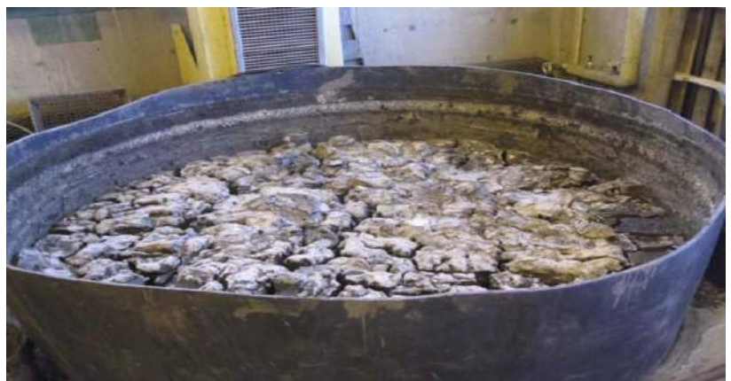
Figure 4. Photographs depicting the processing of Titanium’s fine fluid tailings in a thickener and rim ditch process at CanmetENERGY’s tailings testing facility.
